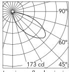
Luminous flux luminaire 543 lm
