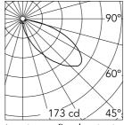
Luminous flux luminaire 543 lm
