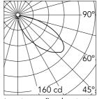
Luminous flux luminaire 503 lm
