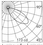
Luminous flux luminaire 543 lm
