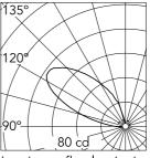
Luminous flux luminaire 260 lm
