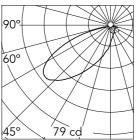
Luminous flux luminaire 260 lm
