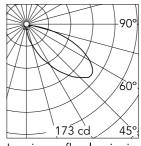
Luminous flux luminaire 543 lm
