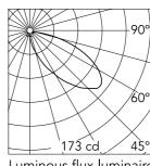
45° Beam Angle: h(m) E(Ix) D(m) 173 2.68 1 2 5.36 43 3 19 8.04 4 11 10.71 5 7 13.39
