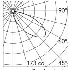
Luminous flux luminaire 543 lm
