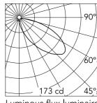
45° Beam Angle: h(m) E(Ix) D(m) 173 2.68 1 2 5.36 43 3 19 8.04 4 11 10.71 5 7 13.39
