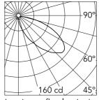
Luminous flux luminaire 503 lm
