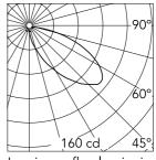
Luminous flux luminaire 503 lm
