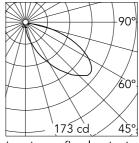
Luminous flux luminaire 543 lm
