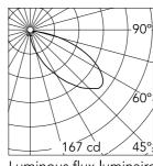
45° Beam Angle: h(m) E(Ix) D(m) 167 2.68 1 2 5.36 42 3 19 8.04 4 10 10.71 5 7 13.39
