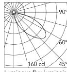
45° Beam Angle: h(m) E(Ix) D(m) 160 2.68 1 2 5.36 40 3 18 8.04 4 10 10.71 5 6 13.39
