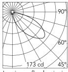
Luminous flux luminaire 543 lm
