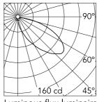
Luminous flux luminaire 503 lm
