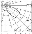
Luminous flux luminaire 503 lm
