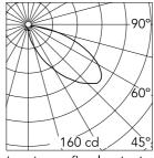
Luminous flux luminaire 503 lm
