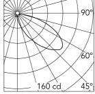
Luminous flux luminaire 503 lm
