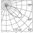
Luminous flux luminaire 543 lm
