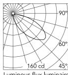
45° Beam Angle: h(m) E(Ix) D(m) 160 2.68 1 2 5.36 40 3 18 8.04 4 10 10.71 5 6 13.39
