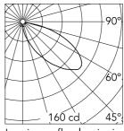
Luminous flux luminaire 503 lm
