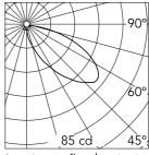
Luminous flux luminaire 266 lm
