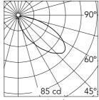
Luminous flux luminaire 266 lm
