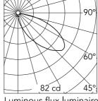
Luminous flux luminaire 256 lm
