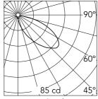
Luminous flux luminaire 266 lm
