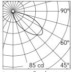
Luminous flux luminaire 266 lm
