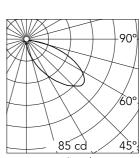
Beam Angle: 45° E(Ix) D(m) h(m) 85 2.68 1 2 21 5.36 3 9 8.04 4 5 10.71 5 3 13.39
