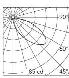
Beam Angle: 45° h(m) E(Ix) D(m) 85 2.68 1 2 21 5.36 3 9 8.04 4 5 10.71 5 3 13.39
