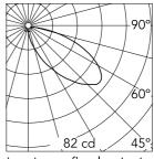
Luminous flux luminaire 256 lm
