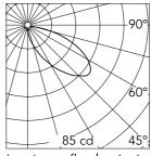
Luminous flux luminaire 266 lm
