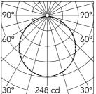
Luminous flux luminaire 667 lm
