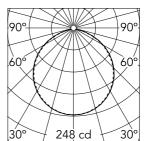
Luminous flux luminaire 667 lm
