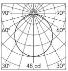
Luminous flux luminaire 124 lm
