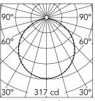
Luminous flux luminaire 855 lm
