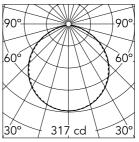
Luminous flux luminaire 855 lm
