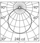
Luminous flux luminaire 667 lm
