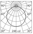
Luminous flux luminaire 667 lm
