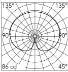
Luminous flux luminaire 1400 lm
