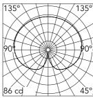
Luminous flux luminaire 1400 lm
