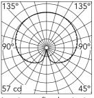
Luminous flux luminaire 700 lm
