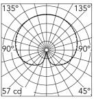
Luminous flux luminaire 700 lm
