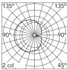
Luminous flux luminaire 423 lm
