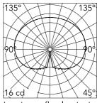
Luminous flux luminaire 192 lm
