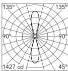
Luminous flux luminaire 796 lm
