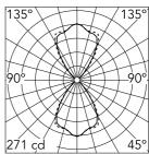
Luminous flux luminaire 708 lm
