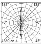
Luminous flux luminaire 779 lm
