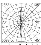
Luminous flux luminaire 909 lm
