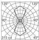
Luminous flux luminaire 825 lm
